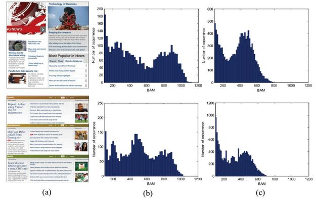
**Fig. 2** BAM histograms of sample SCIs before and after naturalization. (a) Two SCIs; (b) original BAM histograms; (c) BAM histograms after applying the proposed naturalization.
