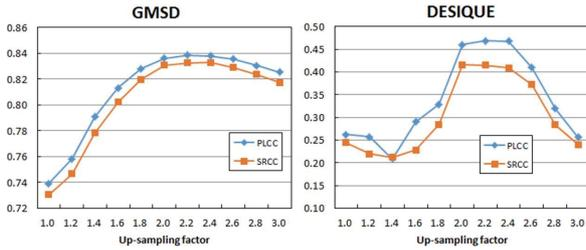
Fig. 3 Impact of up-sampling factors on the metric performances.
