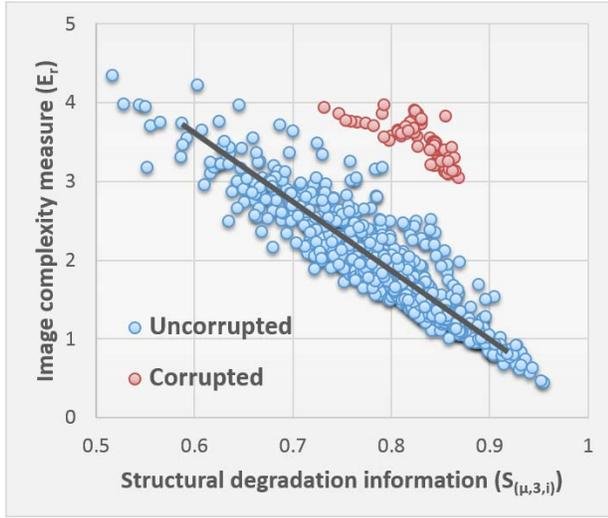
Fig. 6. Representative scatter plot of image complexity feature  $E_r$  versus structural degradation information  $S_{(\mu,3,i)}$  on uncorrupted (blue points) and corrupted (red points) screen content images.
