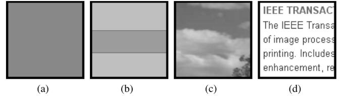
Fig. 4. Comparison of structural degradation information and image complexity measure on four different kinds of image patches: (a) Smooth patch with  $E_r = 0.3916$  and  $S_{(\mu,3,i)} = 0.9975$ ; (b) Edge patch with  $E_r = 0.8021$  and  $S_{(\mu,3,i)} = 0.9868$ ; (c) Textural patch with  $E_r = 2.6455$  and  $S_{(\mu,3,i)} = 0.9808$ ; (d) Textual patch with  $E_r = 3.0838$  and  $S_{(\mu,3,i)} = 0.9077$ .
